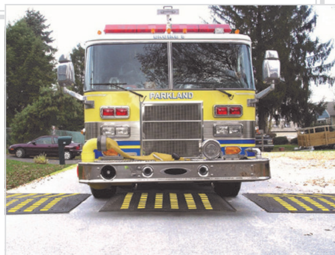
Speed management countermeasures for residential streets may include speed cushions like these, which calm vehicle traffic but include wheel cutouts that allow fire apparatuses to bypass in case of emergency response.
