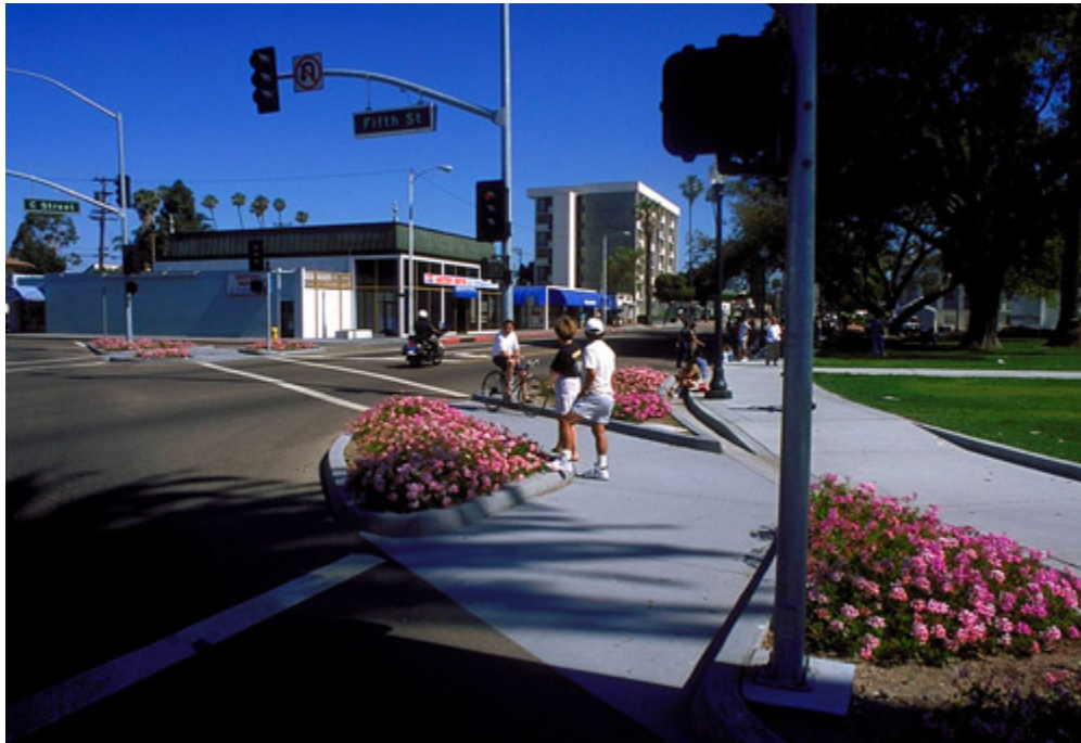
Figure 17. Reduced corner radius at an intersection. Note the location of the previous curb which allowed for higher speed turns by vehicles and increased the crossing distance of the street for pedestrians.
